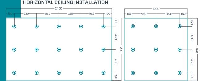
Minimum layout of fasteners 50mm x 1200 x 2400mm sheet.
